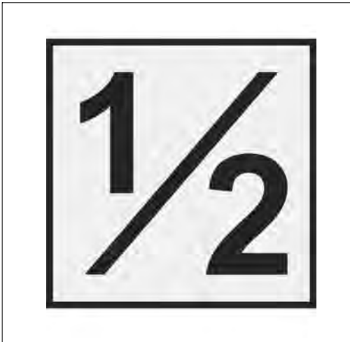
FIG 7-5-1 Typical Runway Half-way Sign
