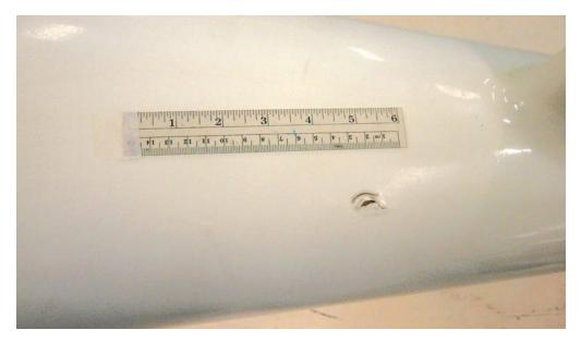
Figure 2-32. Digital image of impact damage.
