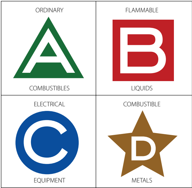
Figure 11-8. Identification of fire extinguisher type location.
