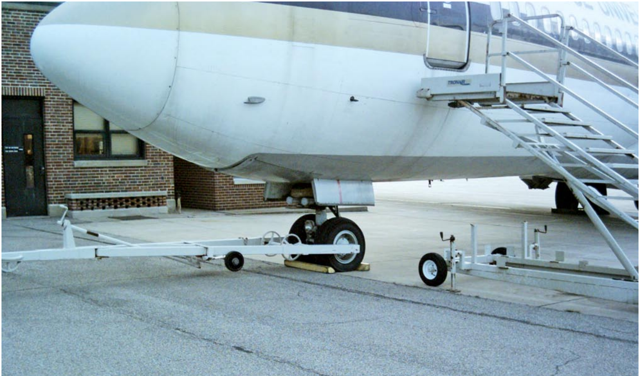
Figure 11-20. Tow bar for a large aircraft.
