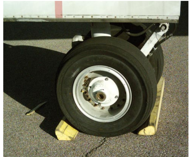
Figure 11-12. Wheels chocked fore and aft.
