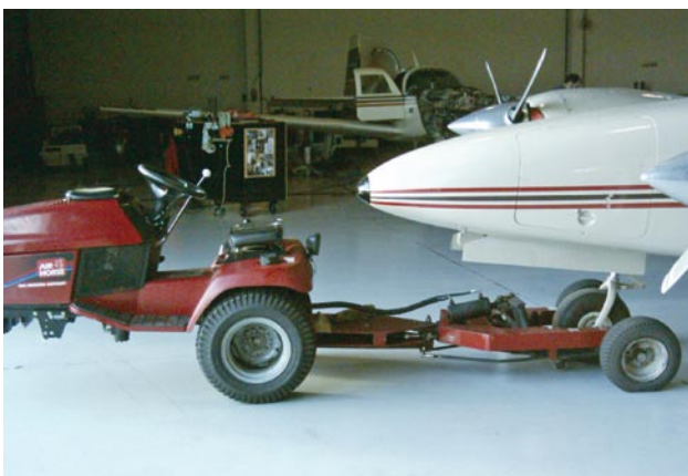
Figure 11-21. Typical smaller aircraft tow tractor.
