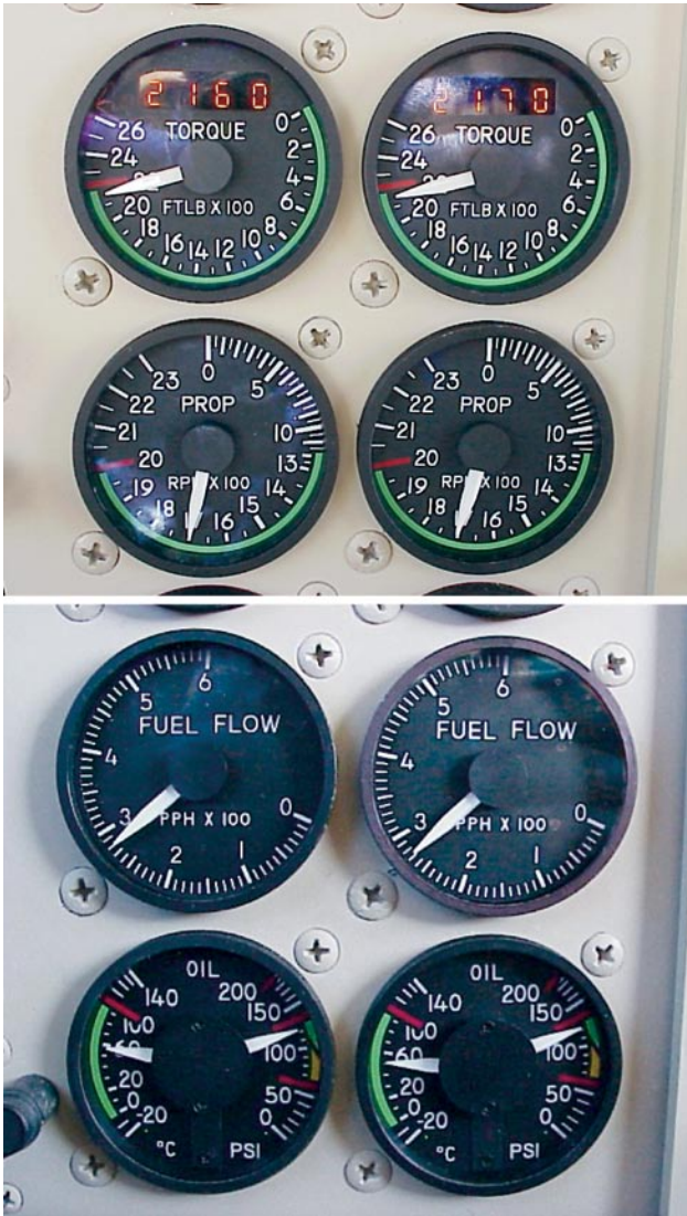
Figure 11-15. Typical examples of turboprop instruments.
