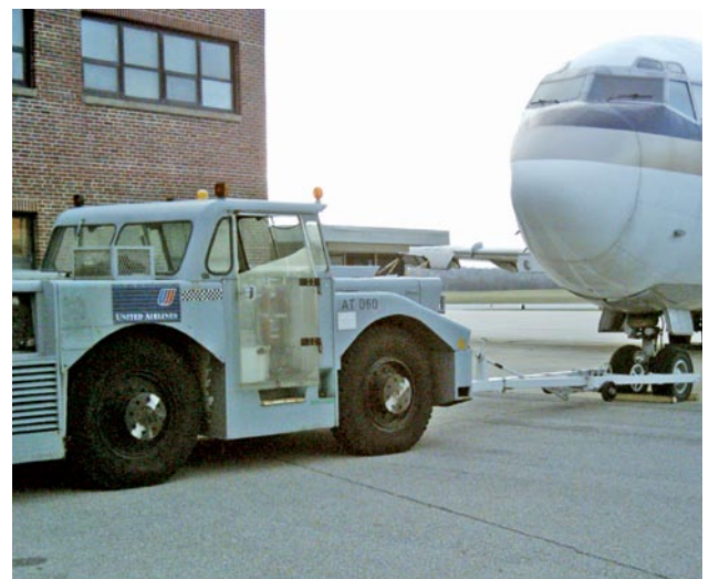
Figure 11-19. Example of a tow tractor.
