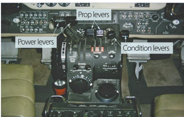
Figure 11-16. Engine controls of a turboprop aircraft.
