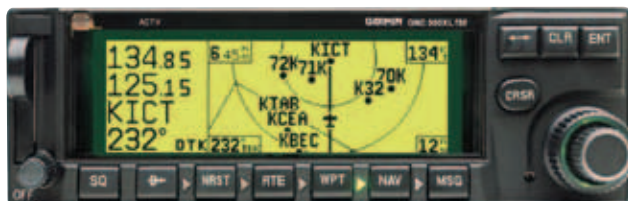
Figure 9-23. Onboard RNAV receivers have changed significantly. Originally, RNAV receivers typically computed combined data from VOR, VORTAC, and/or DME. That is generally not the case now. Today, GPS such as the GNC 300 and the Bendix King KLS 88 LORAN receivers compute waypoints based upon embedded databases and aircraft positional information.
