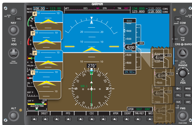
Figure 7-50. Pitch indications for various attitudes (1° through 5°).
