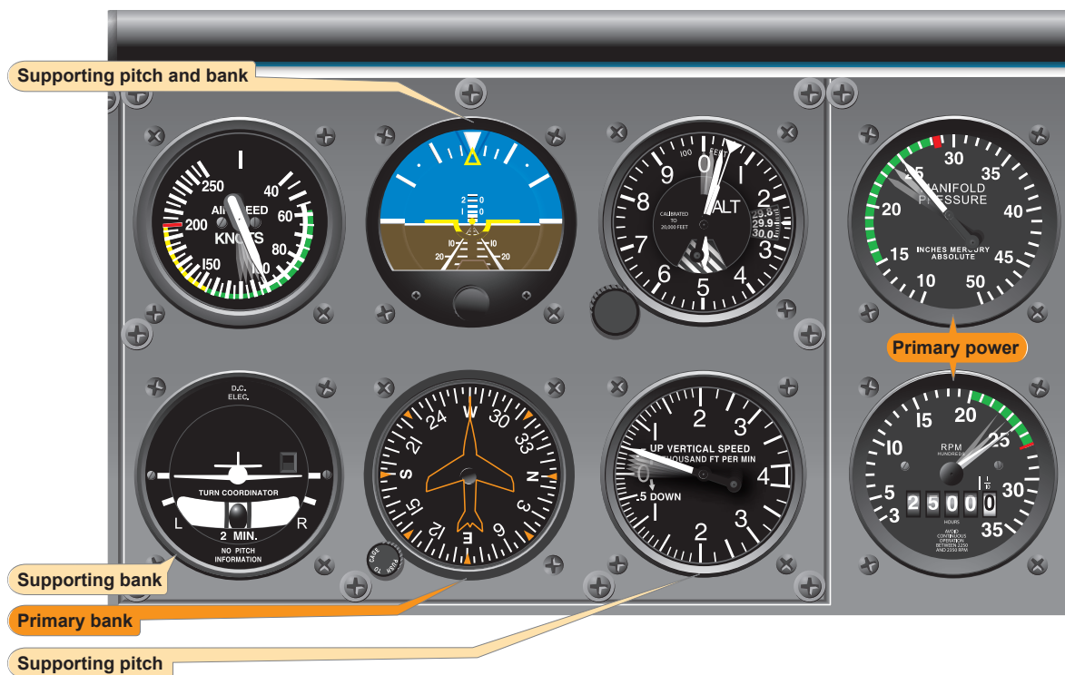
Figure 7-25. Climb entry for constant airspeed climb.
