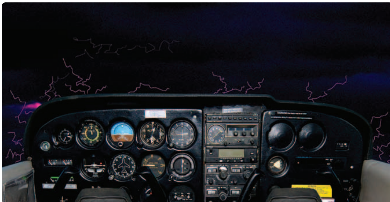
Figure 11-1. St. Elmo's Fire is harmless but may affect both communication and navigation radios, especially the lower frequencies such as those used on the automatic direction finding (ADF).
