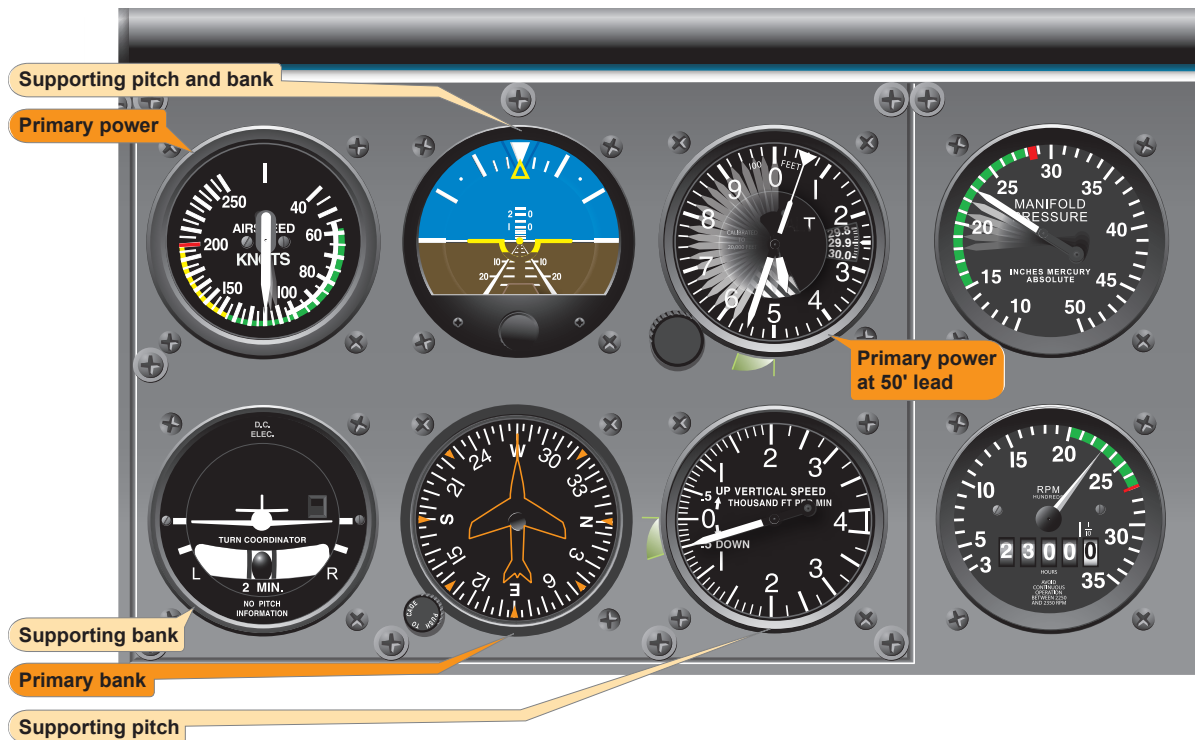
Figure 7-32. Level off at descent airspeed.
