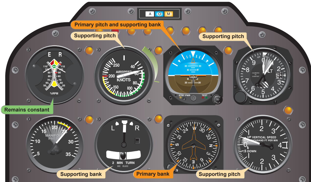
Figure 8-16. Flight instrument indications during an instrument takeoff.
