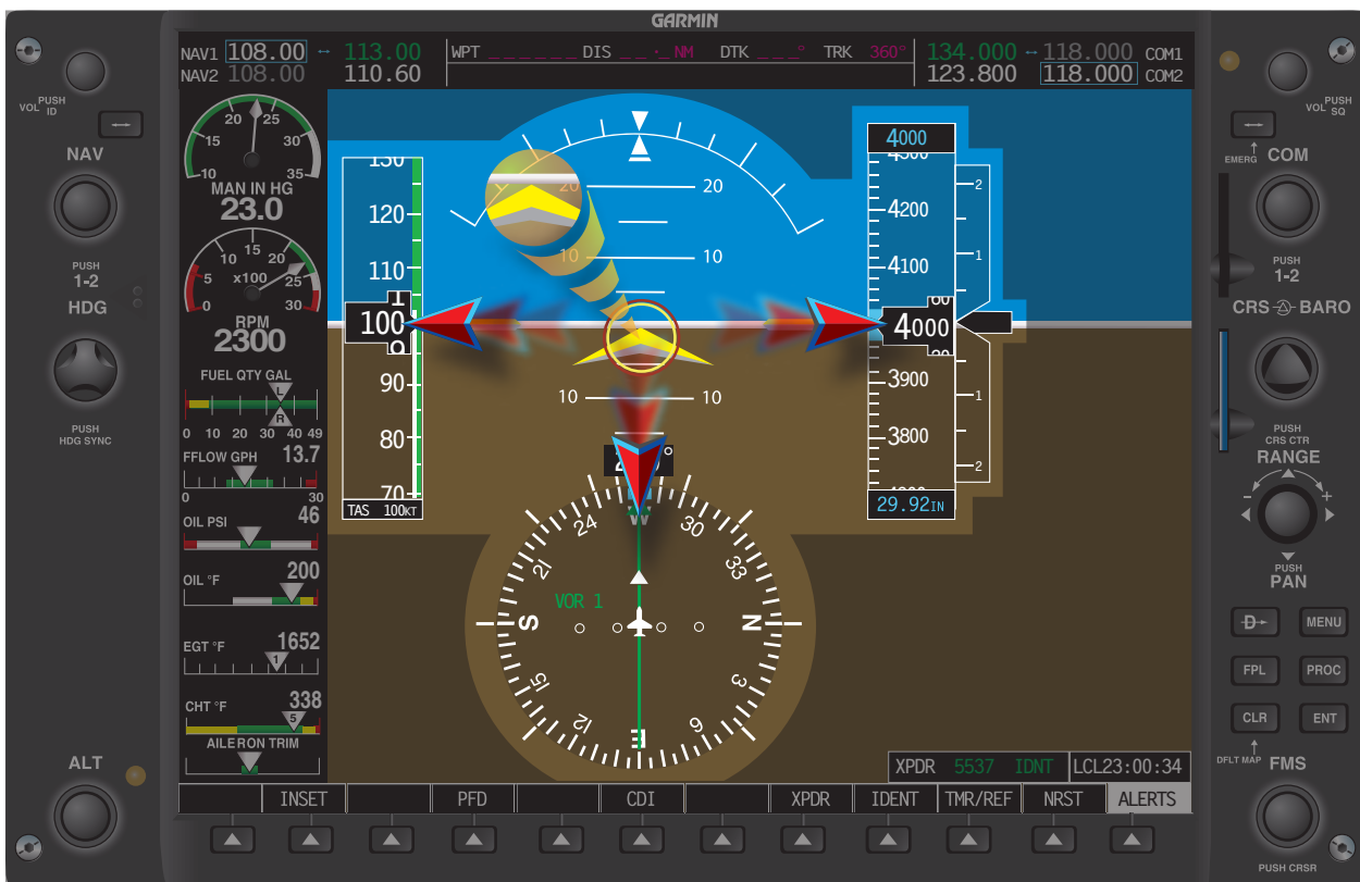
Figure 7-60. Cross-check supporting instruments.
