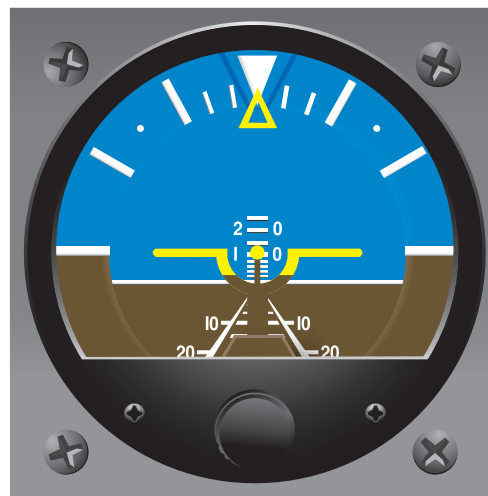
Figure 7-6. Pitch correction for level flight, one-and-one-half bar width.
