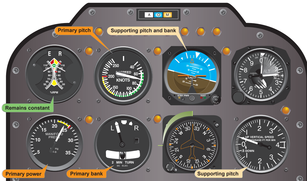
Figure 8-15. Flight instrument indications for a stabilized left climbing turn at a constant airspeed.
