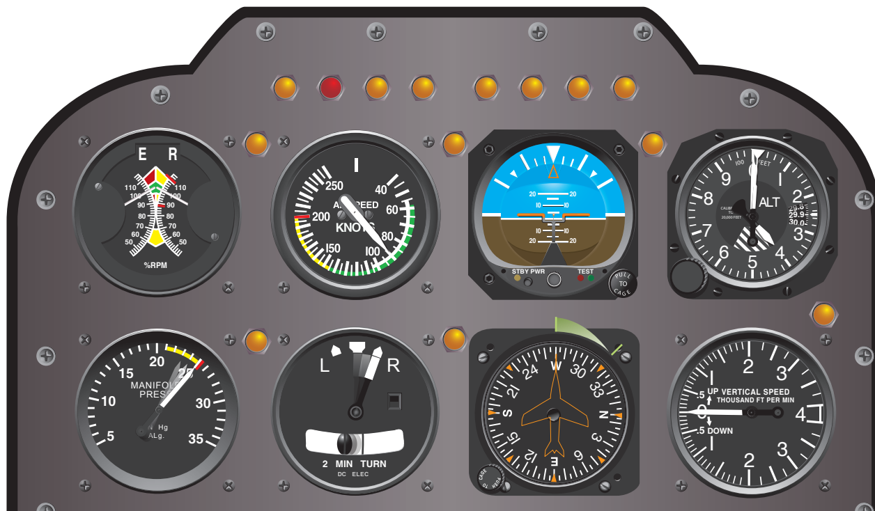
Figure 8-7. Flight instrument indications in straight-and-level flight with power increasing.
