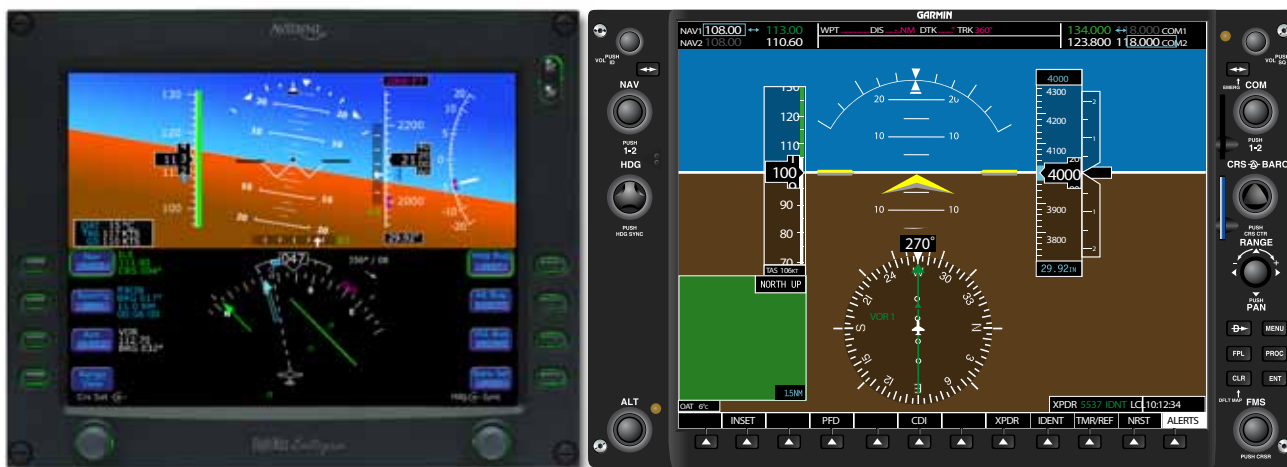
Figure 5-45. Two primary flight displays (Avidyne on the left and Garmin on the right).
