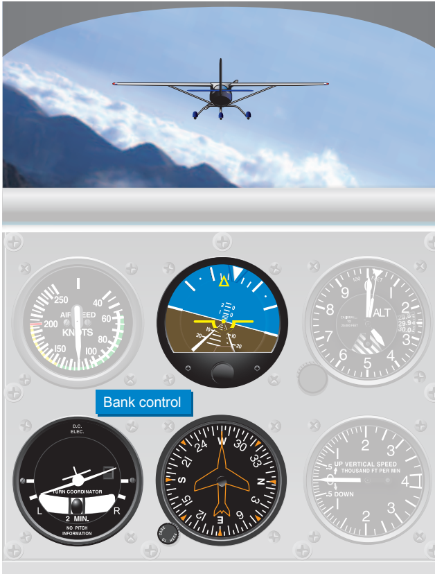
Figure 7-16. Instruments used for bank control.
