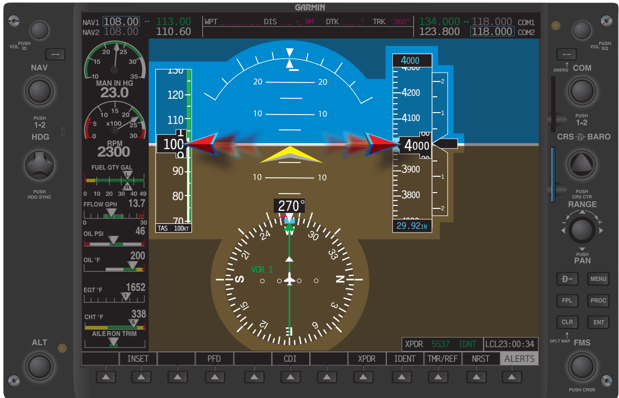
Figure 7-62. The pilot has fixated on pitch and altitude, leaving bank indications unattended. Note the trend line to the left.
