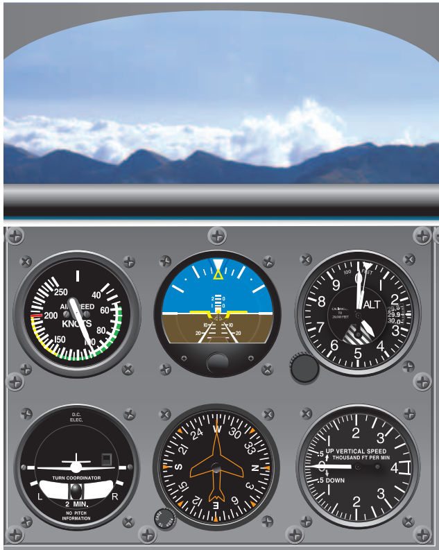
Figure 7-1. Pitch attitude and airspeed in level flight, slow cruise speed.
