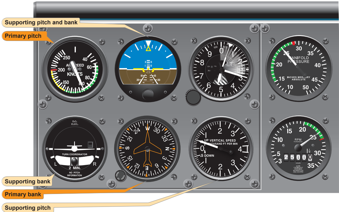
Figure 7-26. Stabilized climb at constant airspeed.
