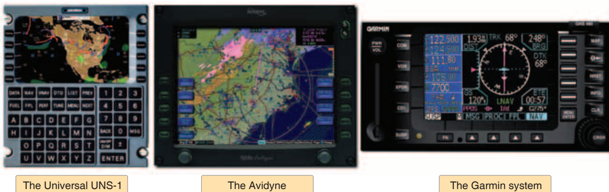
Figure 9-42. Typical display and control unit(s) in general aviation. The Universal UNS-1 (left) controls and integrates all other systems. The Avidyne (center) and Garmin systems (right) illustrate and are typical of completely integrated systems. Although the Universal CDU is not typically found on smaller general aviation aircraft, the difference in capabilities of the CDUs and stand-alone systems is diminishing each year.
