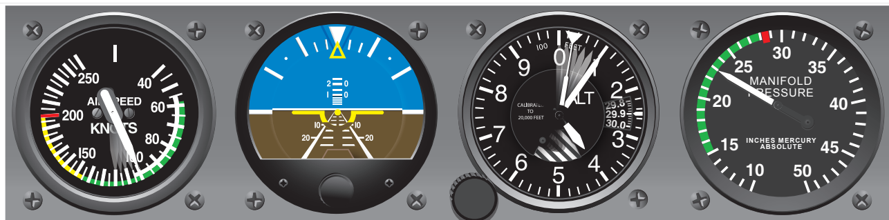
Figure 7-20. Airspeed low and altitude high—lower pitch.
