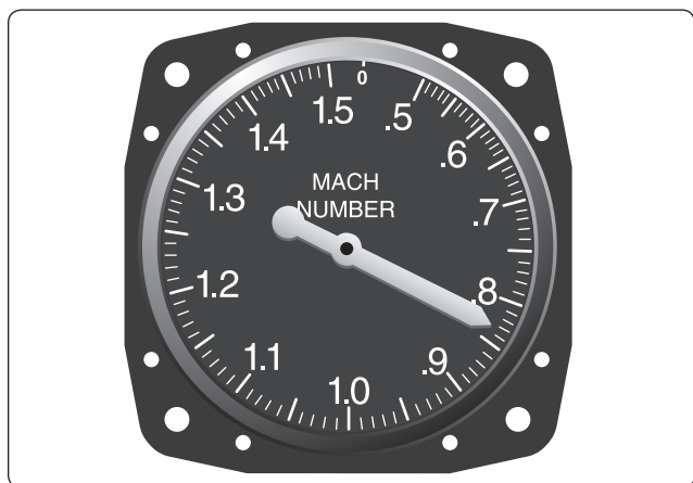
Figure 5-13. A Machmeter shows the ratio of the speed of sound to the TAS the aircraft is flying.
