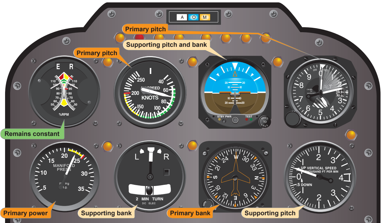
Figure 8-11. Flight instrument indications during climb entry for a constant-air-speed climb.
