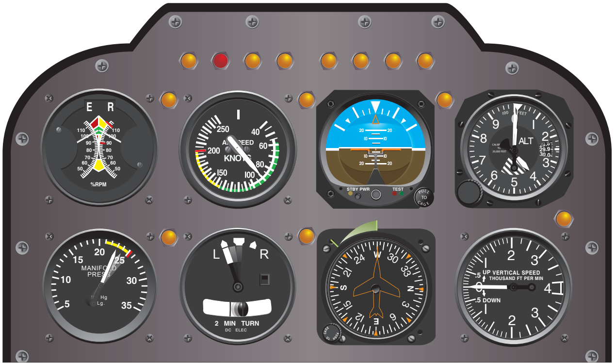
Figure 8-8. Flight instrument indications in straight-and-level flight with power decreasing.
