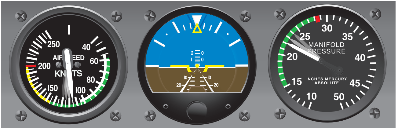
Figure 6-14. Pitch control and power adjustment required to bring aircraft to level flight.
