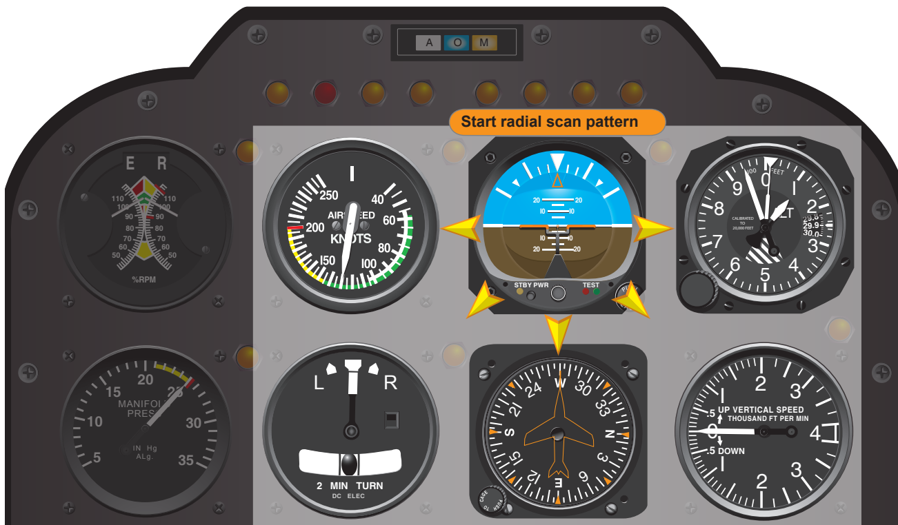
Figure 8-1. A radial scan pattern of the flight instruments enables the helicopter pilot to fully comprehend the condition and direction of the helicopter.
