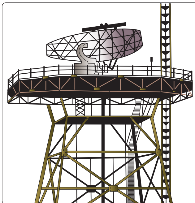
Figure 2-7. Combined radar and beacon antenna.
