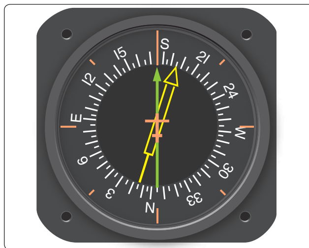
Figure 5-26. Driven by signals from a flux valve, the compass card in this RMI indicates the heading of the aircraft opposite the upper center index mark. The green pointer is driven by the ADF. The yellow pointer is driven by the VOR receiver.
