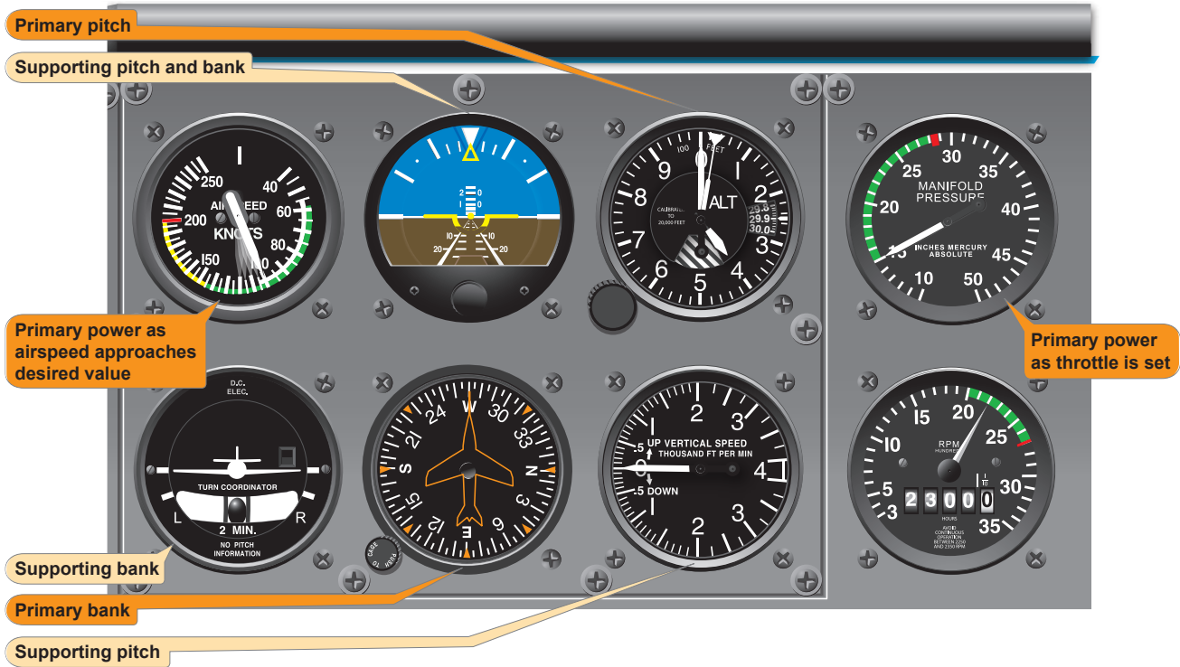
Figure 7-23. Straight-and-level flight (airspeed decreasing).
