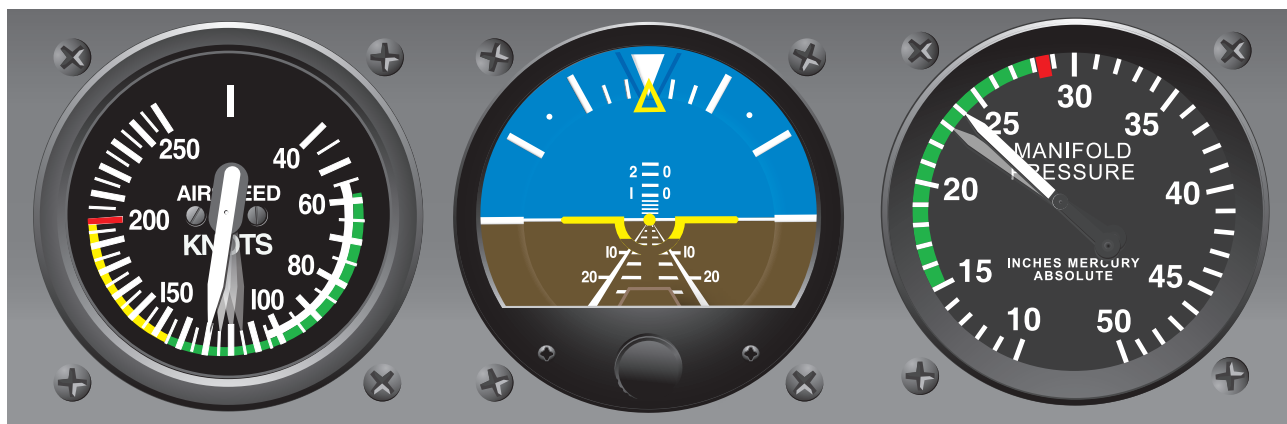
Figure 6-13. An increase in power—increasing airspeed accordingly in level flight.
