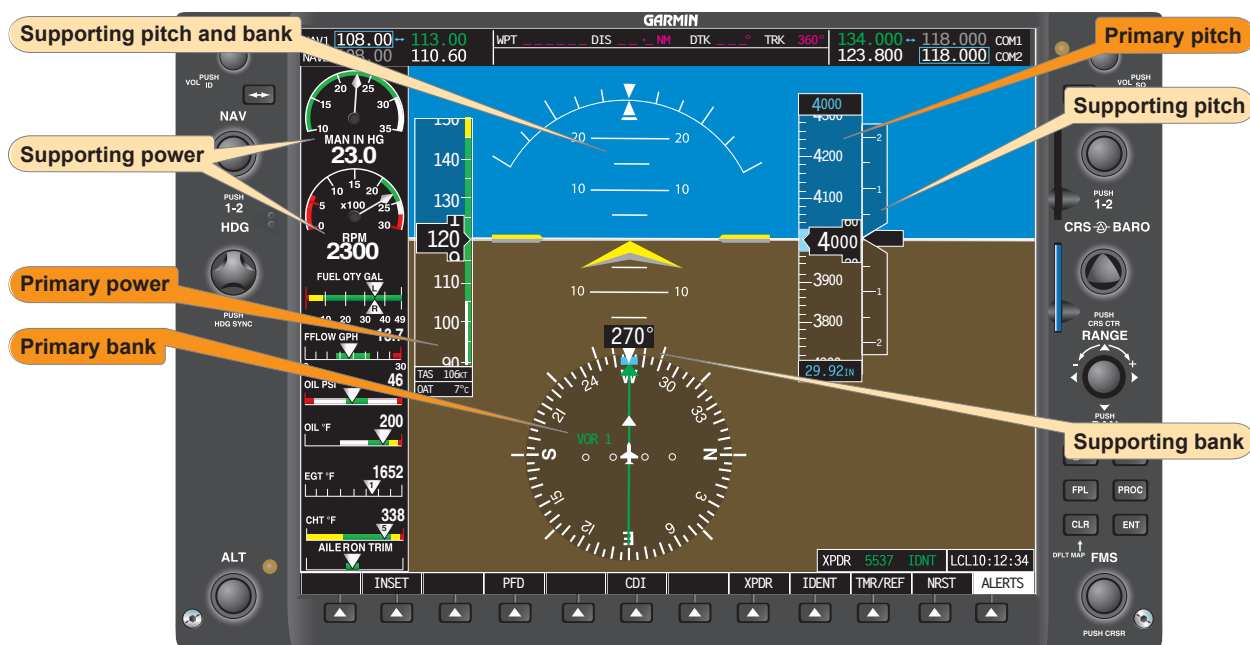
Figure 7-57. Straight-and-level flight (normal cruising speed).
