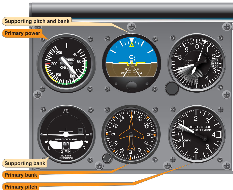
Figure 7-28. Airspeed low and vertical speed high—reduce pitch.
