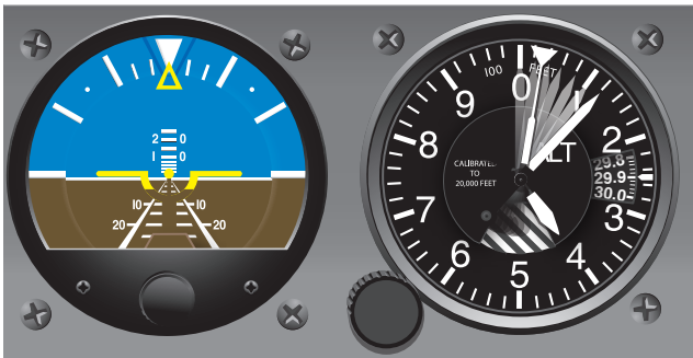
Figure 7-7. Using the altimeter for pitch interpretation, a high altitude means a nose-high pitch attitude.
