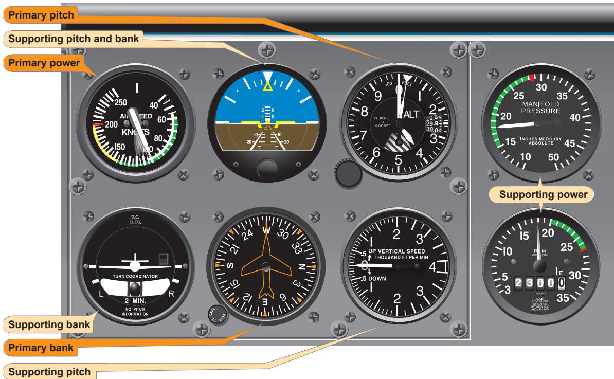
Figure 7-24. Straight-and-level flight (reduced airspeed stabilized).
