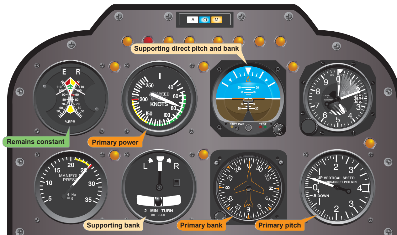
Figure 8-13. Flight instrument indications in a stabilized constant-rate climb.
