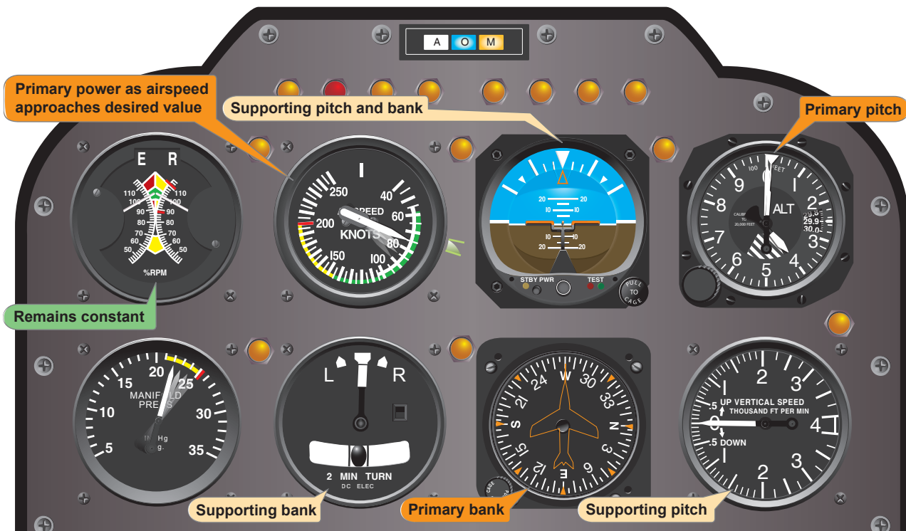
Figure 8-10. Flight instrument indications in straight-and-level flight with airspeed decreasing.
