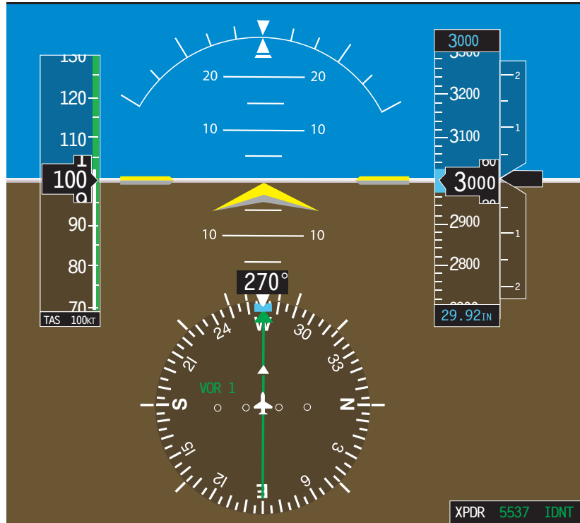
Figure 8-17. PFD indications during straight-and-level flight.
