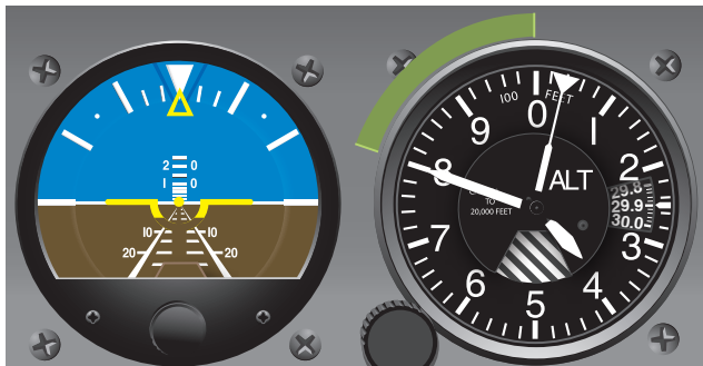
Figure 7-11. Altitude error, greater than 100 feet.
