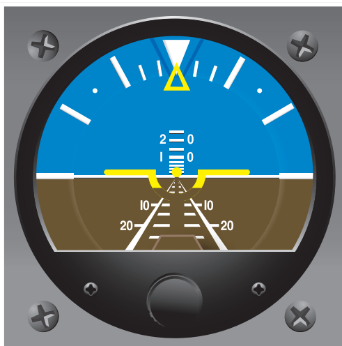
Figure 7-4. Pitch correction for level flight, one-half bar width.
