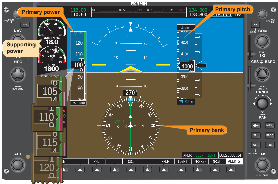
Figure 7-59. Straight-and-level flight (reduced airspeed stabilized).
