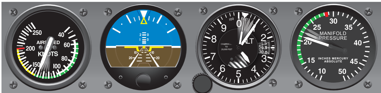
Figure 7-21. Airspeed and altitude high—lower pitch and reduce power.
