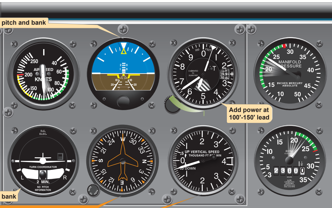
Figure 7-30. Constant airspeed descent, airspeed high—reduce power.
