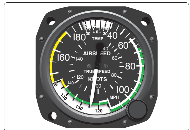
Figure 5-12. A true ASI allows the pilot to correct IAS for nonstandard temperature and pressure.
