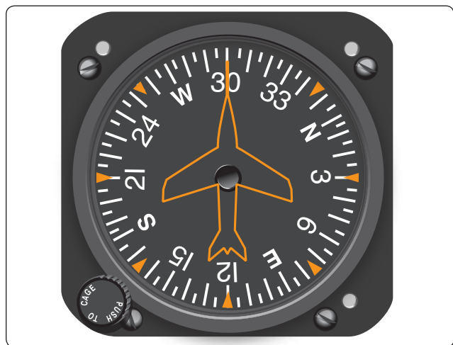
Figure 5-31. The heading indicator is not north seeking, but must be set periodically (about every 15 minutes) to agree with the magnetic compass.
