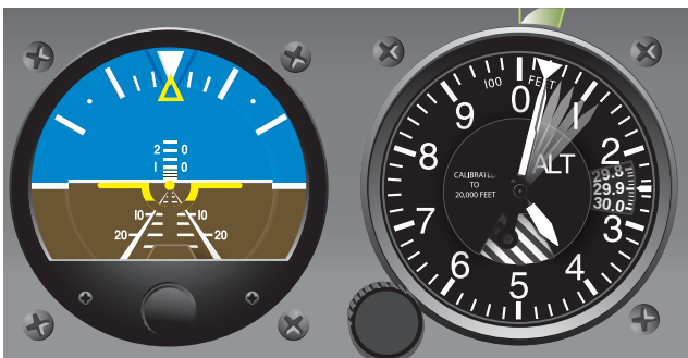
Figure 7-8. Pitch correction following altitude increase—lower nose to correct altitude error.
