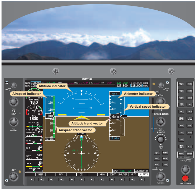
Figure 7-47. Pitch attitude and airspeed in level flight, slow cruise speed.
