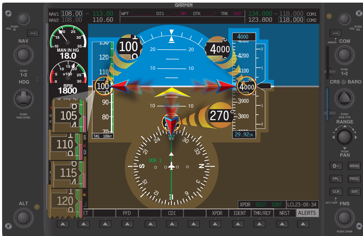
Figure 7-61. Insufficient cross-check. The problem is power and not nose-high. In this case, the pilot decreased pitch inappropriately.
