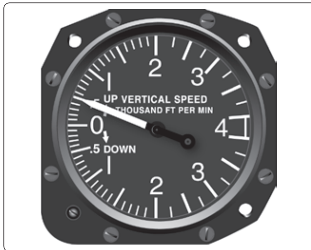
Figure 5-10. Rate of climb or descent in thousands of feet per minute.
