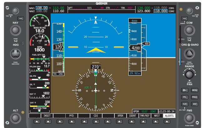
Figure 7-51. Pitch illustrated at 10°.
