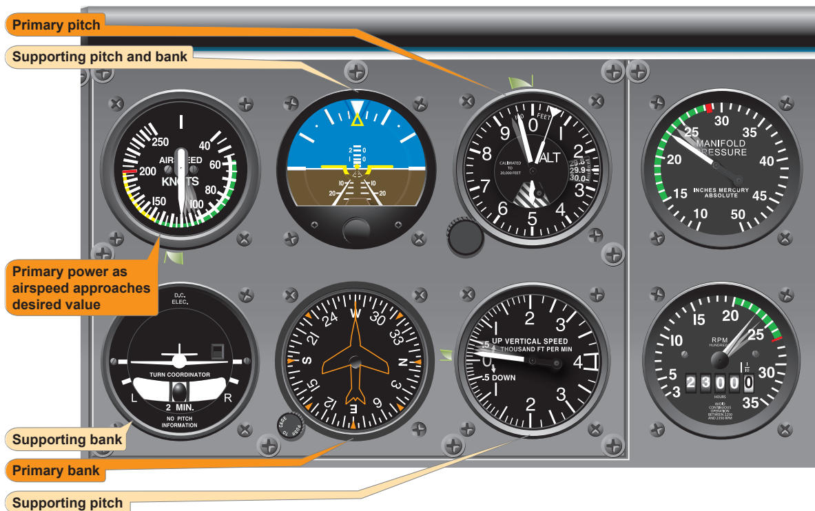
Figure 7-29. Level off at cruising speed.
