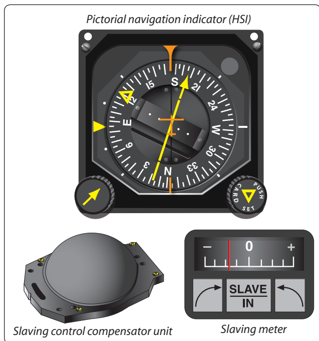
Figure 5-25. The pictorial navigation indicator is commonly referred to as an HSI.
