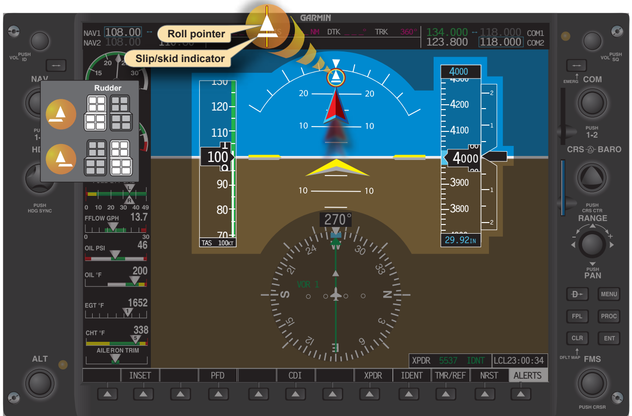
Figure 6-34. Roll pointer and slip/skid indicator.
