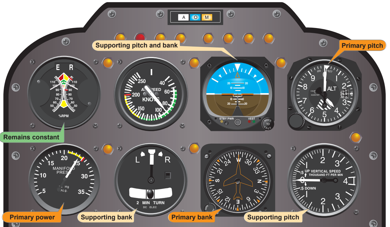
Figure 8-9. Flight instrument indications in straight-and-level flight at normal cruise speed.
