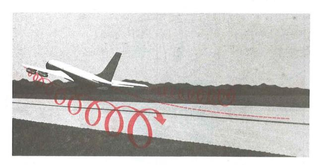
FIGURE 87. Wake turbulence wing tip vortices developing as aircraft breaks ground. These vortices develop when the aircraft is rotated into a flying attitude and the wings begin developing lift.
